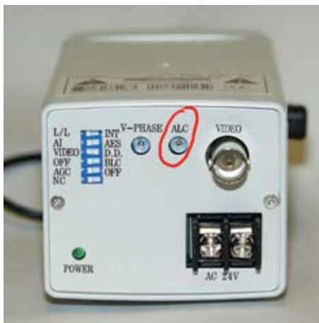
Fig.23 Lens Level is sometimes called ALC
