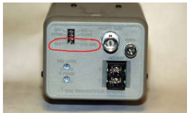
Fig.25 CCD iris is the same as electronic shutter
