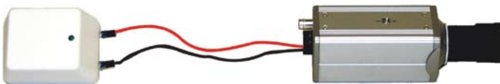
Fig.53 A 24VAC camera powered by a transformer
