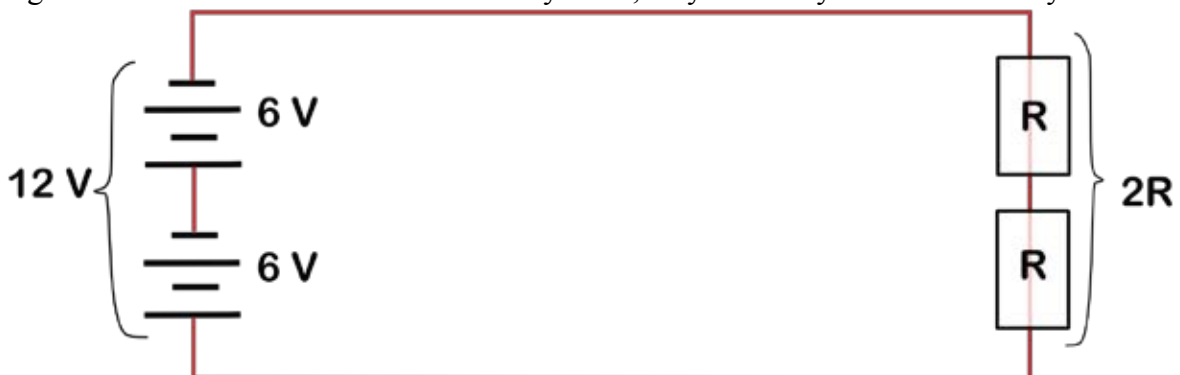
Fig.57 Serial connections of power and serial loading
