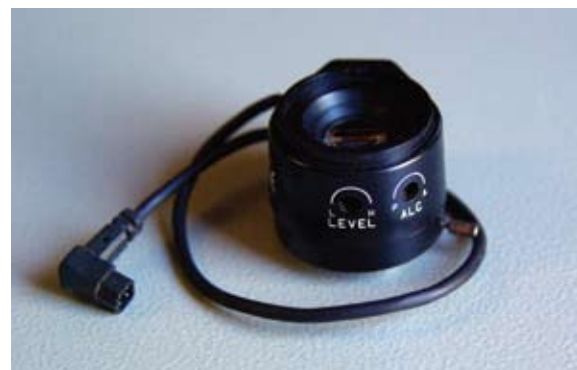
Fig.22 Light level adjustment on video lens
