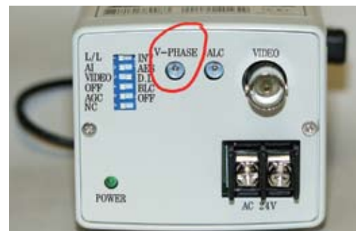
Fig.18 V-Phase works only when LL is On
