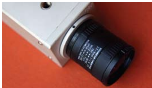
Fig.8 A typical CCTV camera with a manual-iris, vari-focal lens
