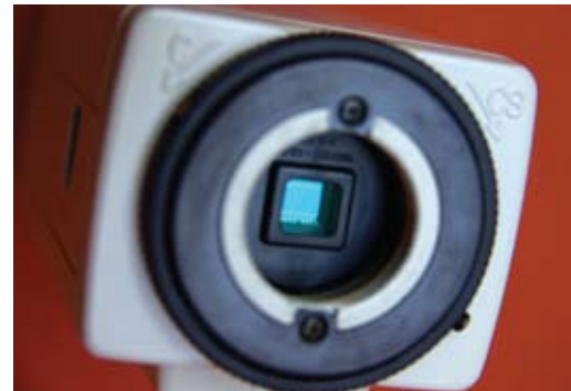
Fig.20 Some cameras can be switched between C and CS-mount
