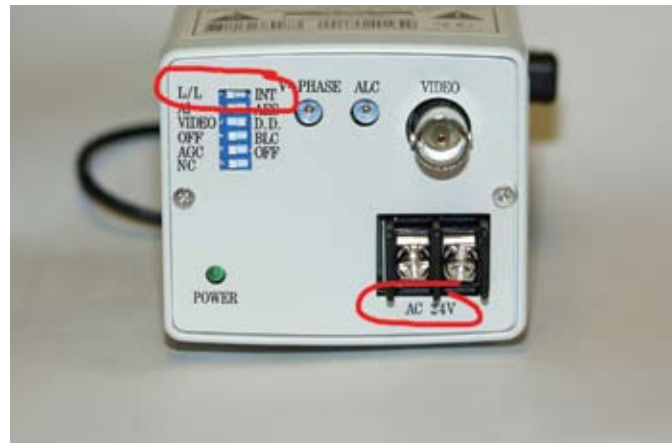
Fig.16 LL can be switched Off or On
