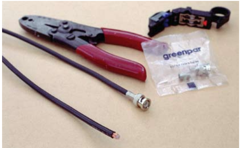
Fig.79 Important for quality: Crimping and stripping BNC tools
