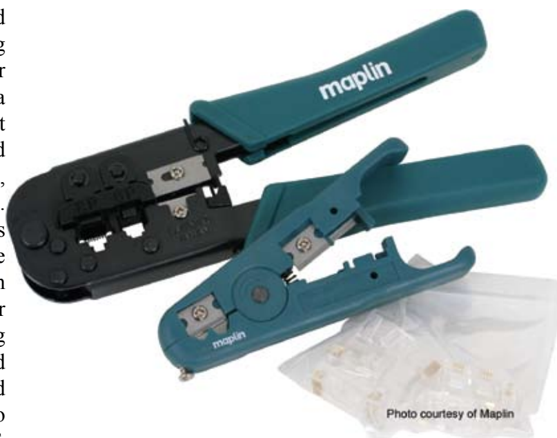
Fig.86 Other tools for terminating Cat cables
