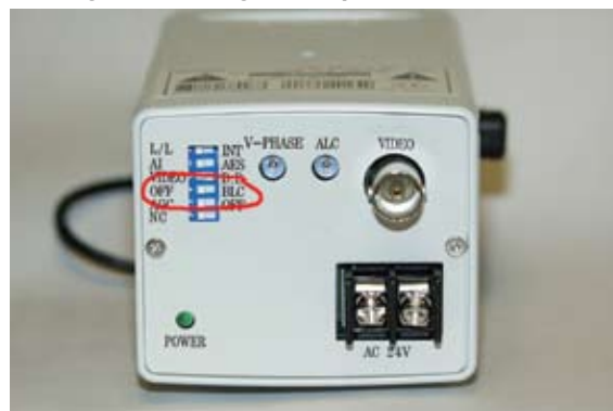
Fig.28 BLC is normally indoor looking out
