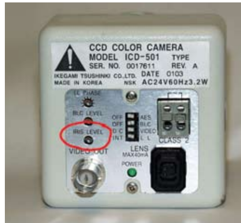
Fig.24 Level only works with DC driven lenses
