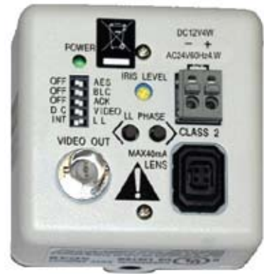
Fig.62 Camera power consumption details
