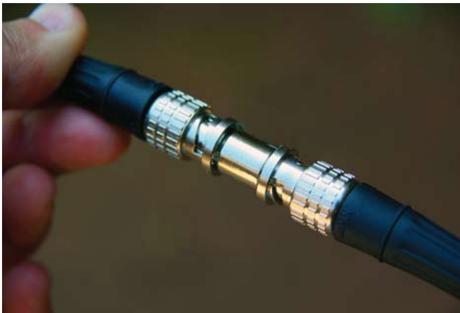
Fig.67 Rubber sleeves help prevent oxidation and sharp bending
