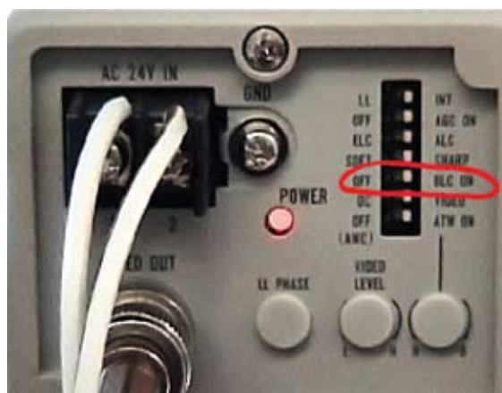
Fig.27 Back Light Compensation Switch
