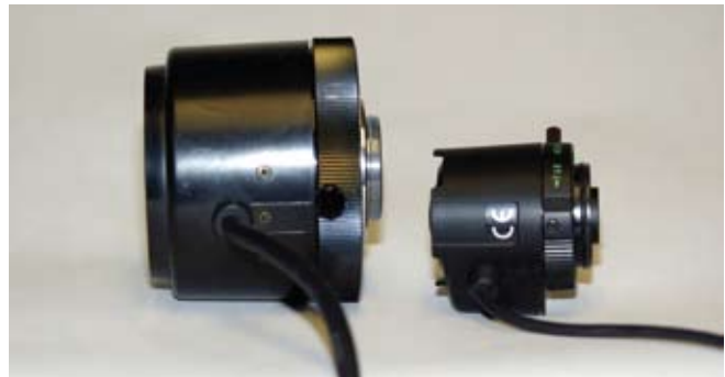
Fig.40 Left, a lens for 1” camera, right for 1/3”
