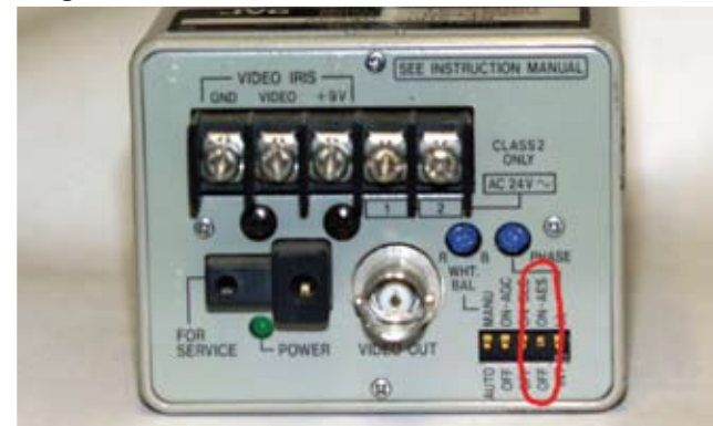
Fig.26 AES should be ON with manual iris lenses
