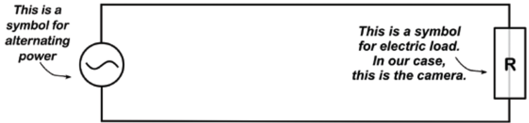
Fig.54 An electric circuit symbolizing the connection on Fig.51
