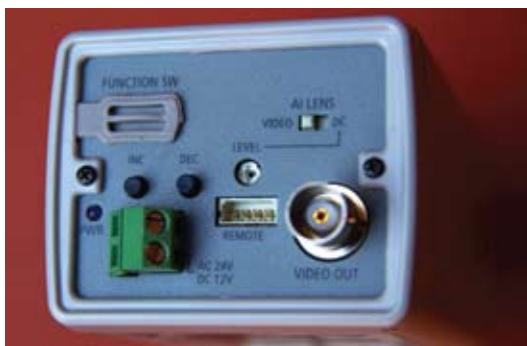
Fig.17 Some cameras can accept both 24VAC and 12VDC power
