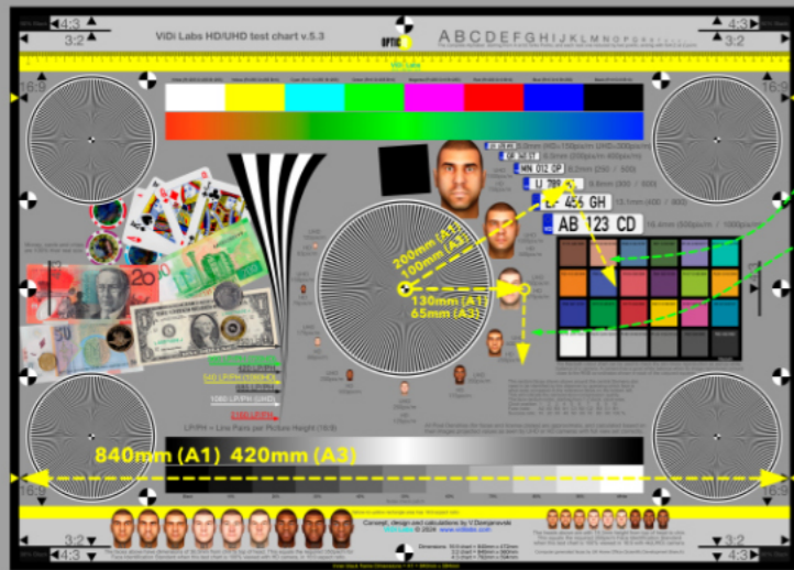
The raw electronic version of the test chart with the random faces around the clock representing various pixel densities and the various size number-plates in the top-right hand quadrant
